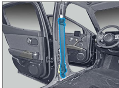
1) Front Seatbelt Pretensioner
